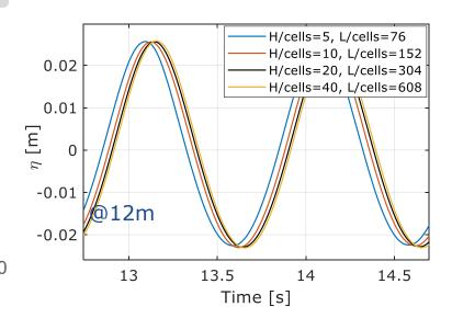
□ For H/cells=20 and L/cells=304, error on H<5% and phase difference <0.1s
