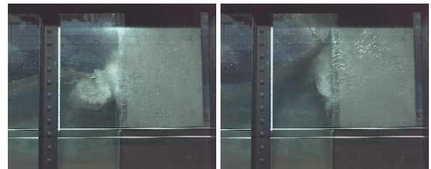
Figure 2 - Trapped air between wave front and wall
