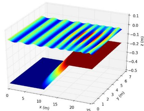
Figure 1 - Bathymetry of the experiments of Whalin (1971) and snapshot of the simulated free surface elevation.
