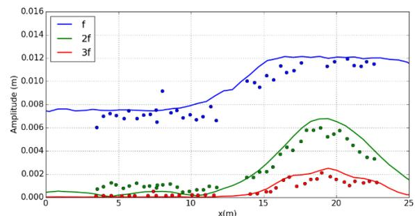
Figure 2 - Simulated (solid line) and measured (dots) harmonic amplitudes along the center axis of the basin of the experiment of Whalin (1971) with  $T = 2$  s and  $A = 7.5$  mm.
