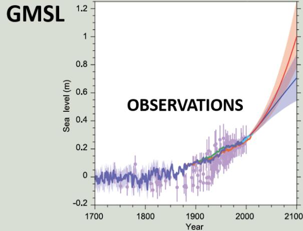
**TFE.2, Figure 2** | Compilation of paleo sealevel data (purple), tide gauge data (blue, red and green), altimeter data (light blue) and central estimates and likely ranges for projections of global mean sea level rise from the combination of CMIP5 and process-based models for RCP2.6 (blue) and RCP8.5 (red) scenarios, all relative to pre-industrial values. (Figures 13.3, 13.11, 13.27)
