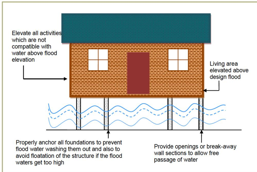
Figure 4.22: Basic dry flood-proofing measures for a residential structure
