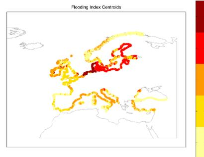
$$\text{Flooding Index} = \text{Coeff}_{\text{manning}} \times \frac{\text{TWL}_{100\text{YRP}} \times (\alpha_{\text{GOS}} + \alpha_{\text{SETUP}})}{\text{Slope}_{\text{mdt}}}$$
