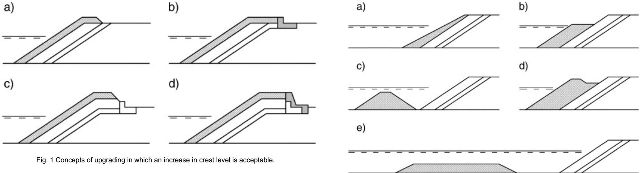
Fig. 1 Concepts of upgrading in which an increase in crest level is acceptable.
