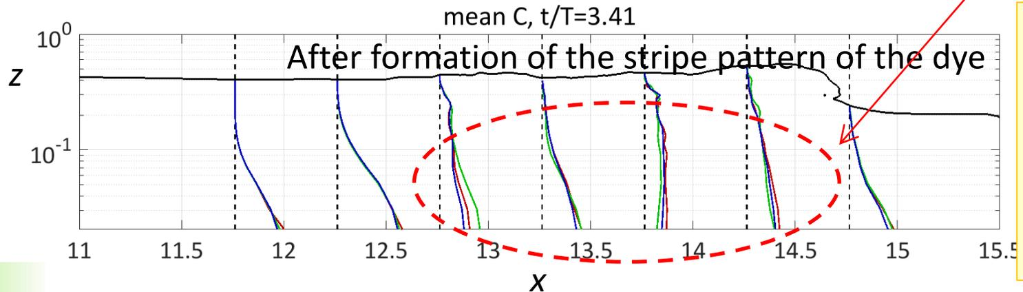
Dye transport mainly driven by advection by structured vortices. Diffusion have a limited effect.
