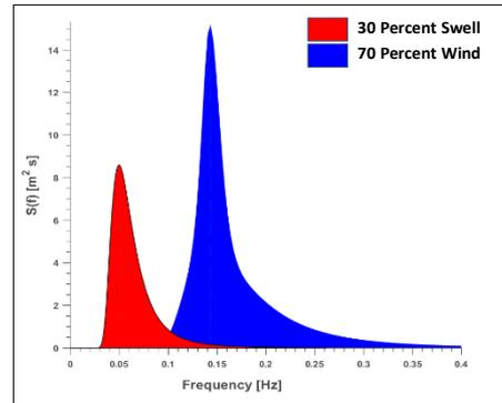
Figure 2: A snapshot of a partitioned 2-D plot of an energy density spectrum partitioned for WC (@70%) and SC (@30%) Train at St Mary's Sound (Channel Coastal Observatory buoy (CCO, 2017), with VM Code 6201053) at 01:00 UTC on December 24, 2014.
