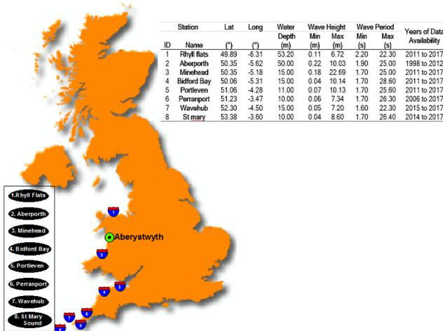
Figure 1 - Descriptions and Geographical Coordinates of Wave Buoy Stations used in the analysis.
