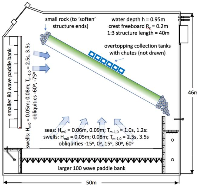
Figure 3: Sketch of the layout of the structure in the Delta Basin. Not to scale.
