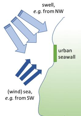
Figure 1: Seawall exposed to crossing sea and swell.
