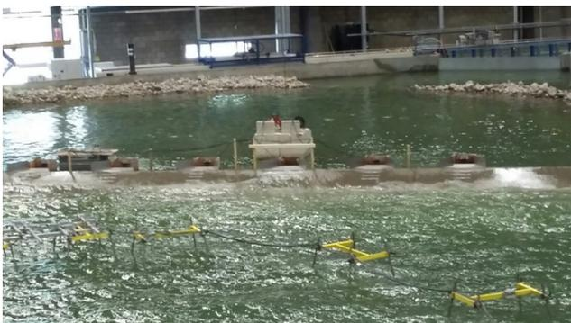
Figure 5: Photograph of testing, showing the six overtopping collection tanks.
