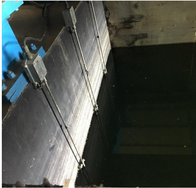
Piston-type absorbing wave maker
