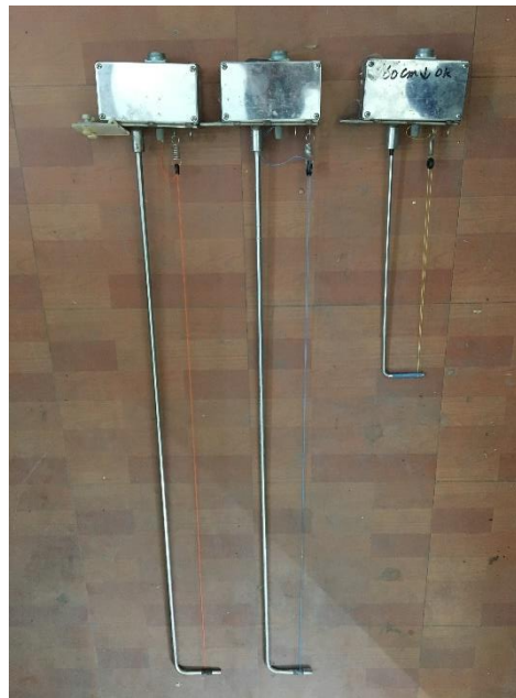
30 wave gauges ( F_s = 100 \text{ Hz} )
