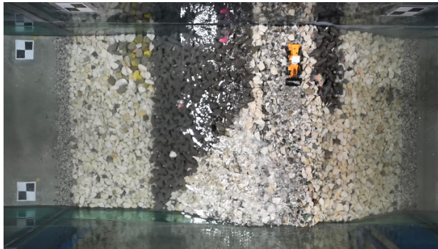
Fig 4. Top view 2D model, tests of structure loaded by a storm during a simulation of the construction phase
