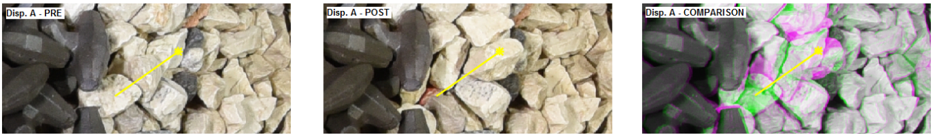
Fig 2. Example of output of the photographic overlay technique to investigate the structure stability
