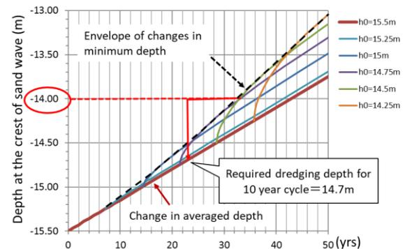
Figure 5 Depth change at the crest of sand wave predicted from critical condition of sand wave formation
