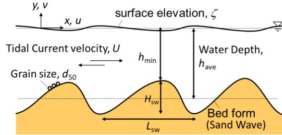
Figure 2 Definition of minimum depth,  $h_{min}$  and averaged depth,  $h_{ave}$  on sand waves
