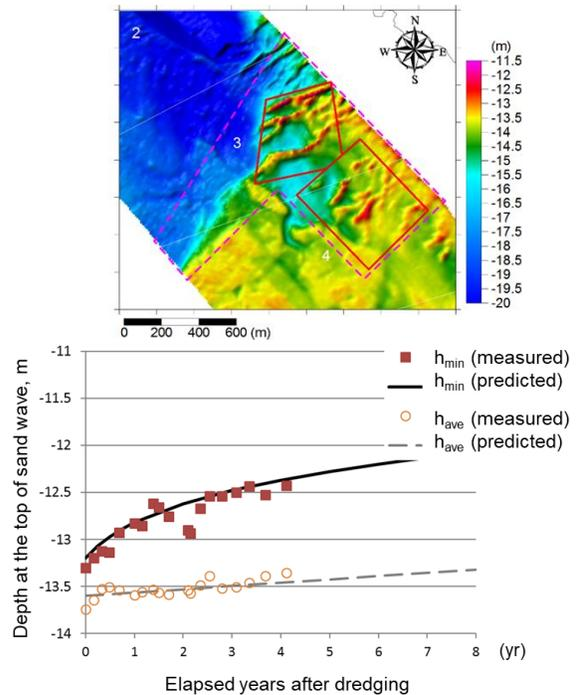
Figure 3 Sea bed topography of Kasase in Kanmon channel (top) and comparison between measured and predicted change in minimum depth (bottom)
