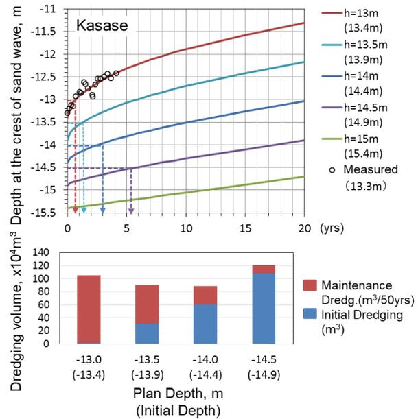
Figure 4 Predicted changes in minimum depth at the crest of sand wave for each plan depth (top), and totally required dredging volume (bottom)
