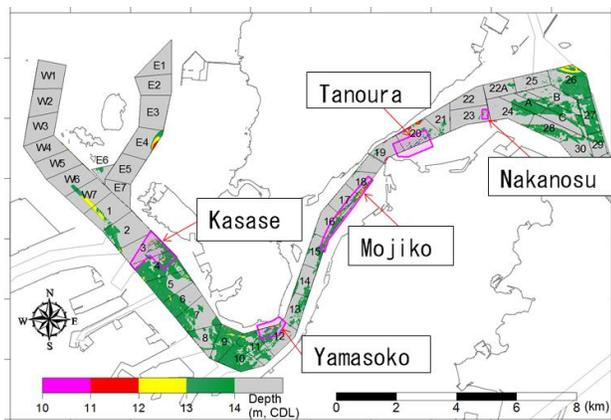
Figure 1 Typical five areas sand waves are formed in Kanmon route, Japan
