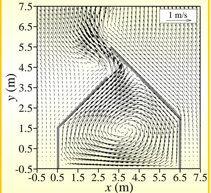
⇒ Flow spreading by numerical diffusion is reduced in the WENO scheme.
