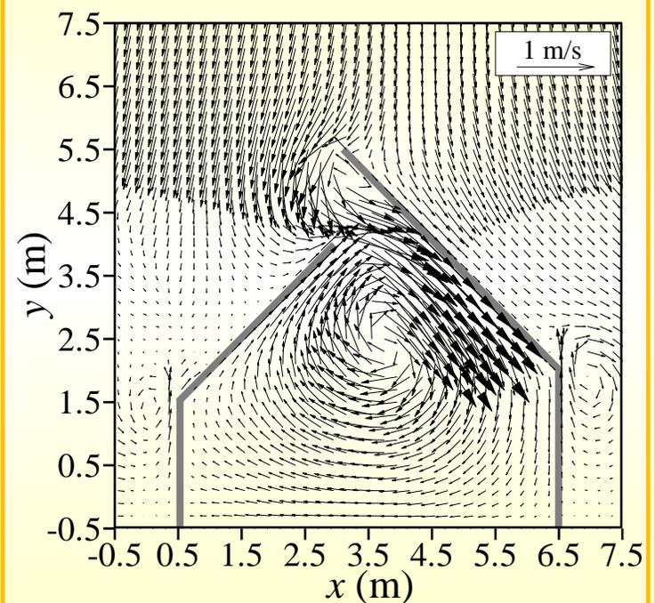
⇒ Calculated flows near breakwaters are reproduced smoothly along the breakwaters by introducing the FAVOR method.
