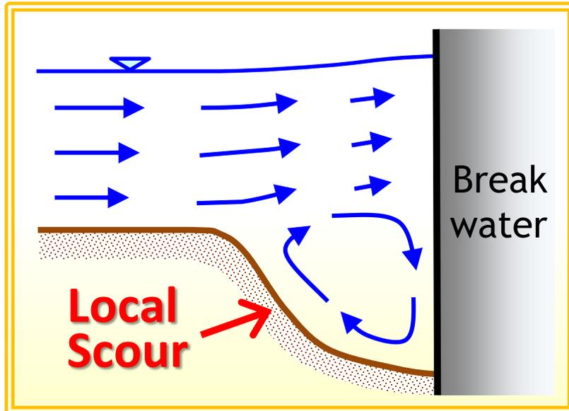
3D flow field is generated around a harbor when tsunami strikes.
