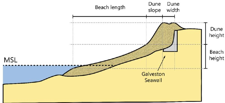
Figure 3. Schematic cross-section of the hybrid setup under consideration. Design parameters that were varied as part of this study are displayed.
