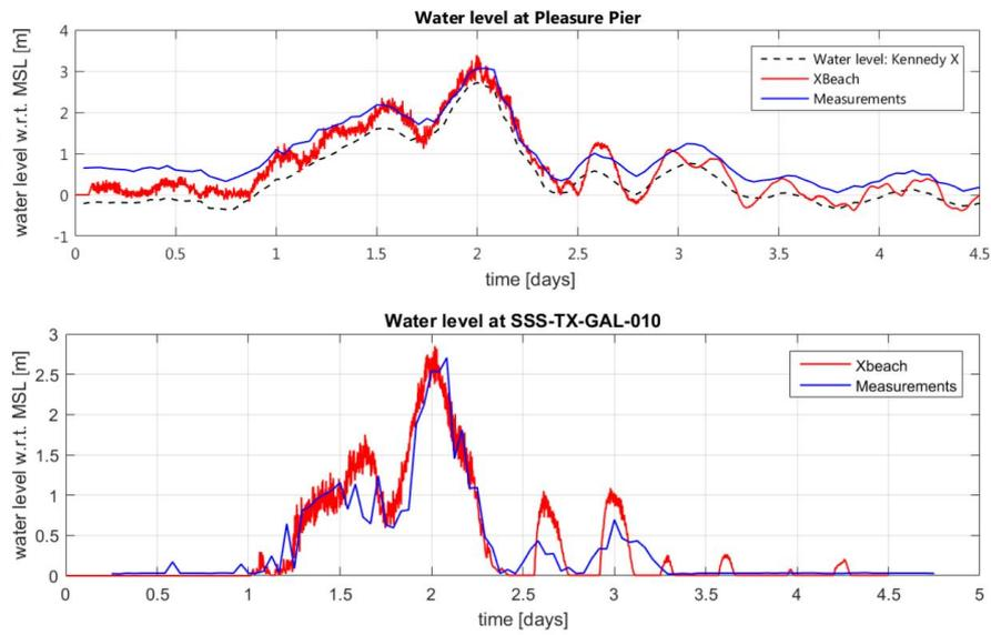
Figure 7. Storm surge validation between predicted (red) and measured (blue) water levels for the Galveston Pleasure Pier tidal gauge (SID: 8771510; 29°17.1'N; 94°47.3'W (NOAA, 2016c)) in front of the GSW (top panel) and at a temporary onland gauge (SID: SSS-TX-GAL-010; 29°14.1'N 94°52.4'W (USGS, 2008)) at the west end of the GSW, where only small dunes are present (bottom panel).
