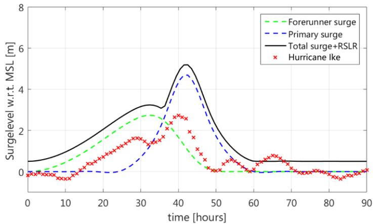
Figure 5. Time series of storm surge level for a 100-year event including forerunner surge (green) and primary surge (blue) (Lendering et al., 2014) and final combined surge level accounting for RSLR (black). Reference is made to measured surge levels during Hurricane Ike at offshore buoy S42035 (NOAA, 2016a).
