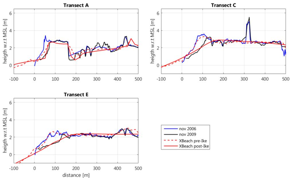
Figure 8. Predicted and measured cross-shore profiles before and after Hurricane Ike impact at the west end of the GSW on Galveston Island. Transect A is located just west of the west end of the GSW and features several non-erodible structures, such as a parking lot and elevated roads. Transects C and E are located westward of transect A and feature only small dune formations. The large elevation in the middle of Transect C represents a man-made structure and was not included in the model.
