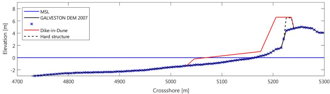
Figure 4. Cross-section of hybrid setup for simulation with run ID 2.10 (see Table 1). In this case GSW is increased to MSL + 6.5 m.
