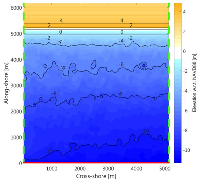
Figure 4. Model domain with initial bathymetry, composed of measured bathymetry offshore and simplified profile behind the seawall. In the initial setup, no sand cover is added and the seawall is exposed. Incoming surge and waves are described at the offshore boundary (red). The lateral boundaries were defined as Neumann boundaries (green).
