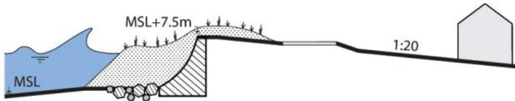
Figure 2. Schematic overview of sand cover over the GSW (Jonkman et. al. 2015).
