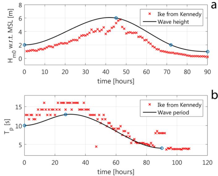
**Figure 6.** Time series of design significant wave height (a) and peak wave period (b) used for the hybrid simulations (black). Reference is made to the measured wave height and period during Hurricane Ike by rapidly deployed buoys in around 10 m water depth along the Upper Texas Coast (Kennedy et al., 2011a).
