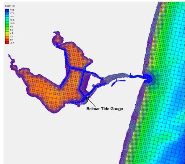
Figure 1 - Computational Mesh for the Shark River Inlet
