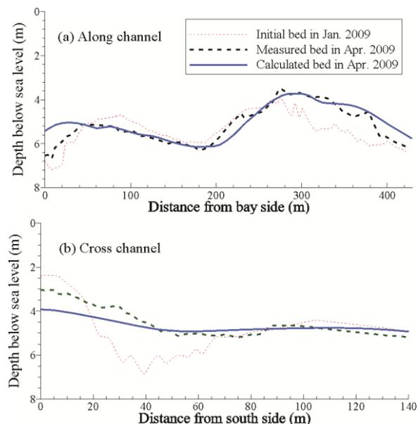
Figure 2 - Measured vs. Calculated Bed Levels
