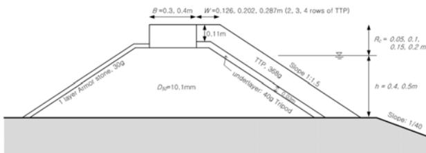
Figure 1 - Schematic sketch of rubble mound structures
