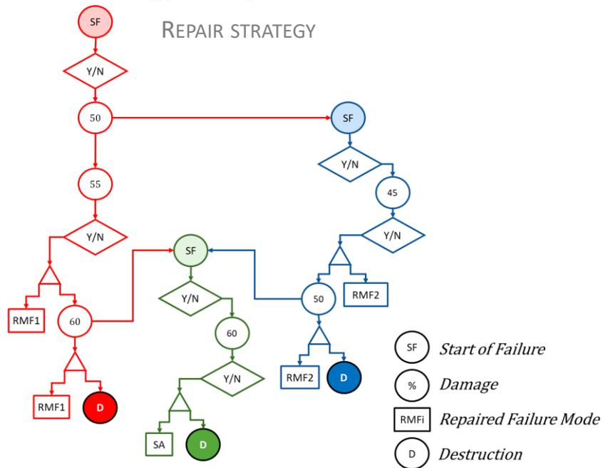
Series failure diagram: breakwater fail when one mode of failure occur
