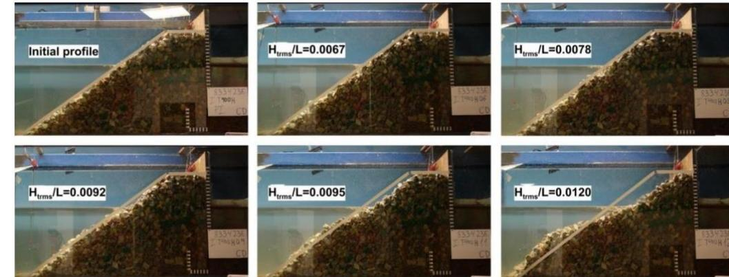
Damage Accumulation Tests in rubble mound breakwater (UGR)
