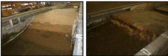
Figure 1 . Dune formation and swash zone instruments (left) and dune face after the storm wave impacts (right)
