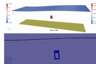
Figure 3. Numerical simulation of waves and current interacting with a floating body using the overset method.
