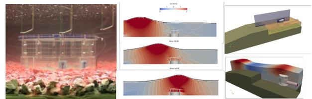
Figure 2. Left panel: experimental set-up. Middle panel: velocity ( $U_x$ ) patterns corresponding to the largest wave passing over the intake structure. Right panel: Numerical domain including buried tower and pipe.
