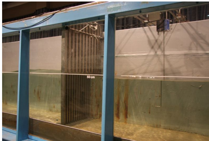
Figure 2. Perforated wall and wave gauges installed in wave flume in KORDI.
