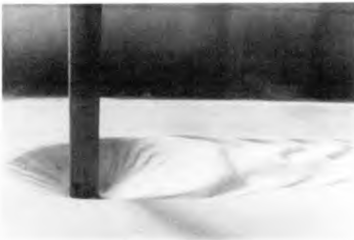
Figure 8. Scour pattern 2 to 3 hours after test commencement.
