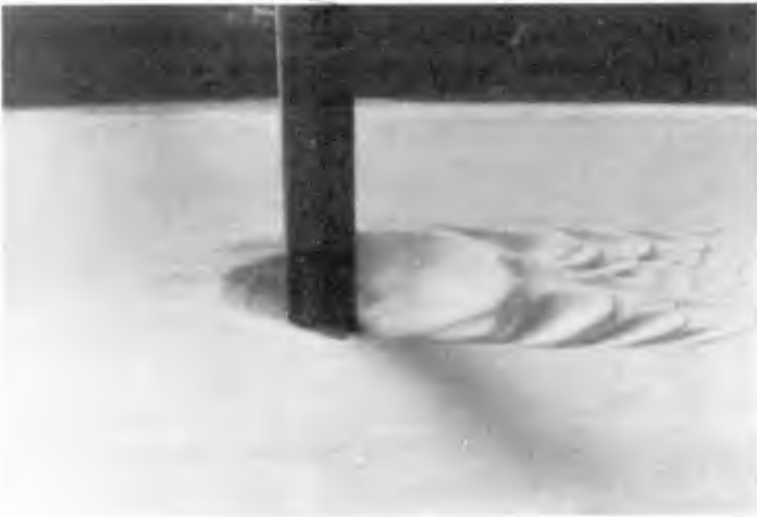
Figure 7. Scour pattern 30 minutes after test commencement.
