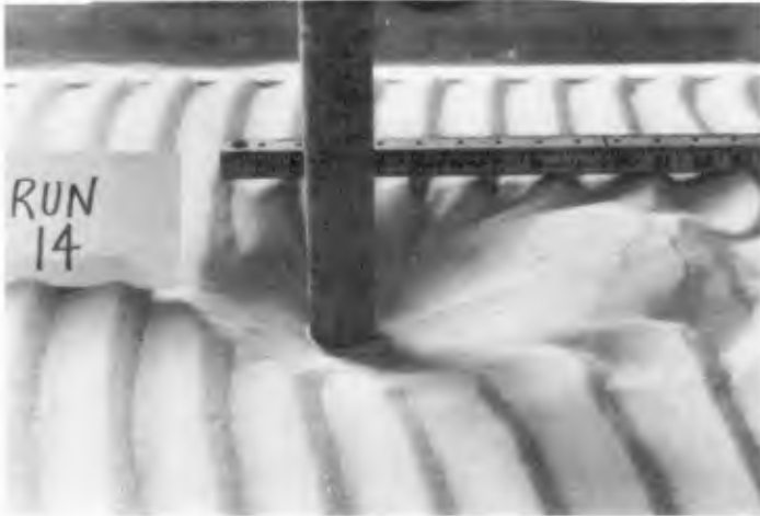
Figure 11. Scour pattern due to random waves and current - Run 14. h=1.167 ft (0.36 m); U_c=.485 ft/sec (0.148 mps); U=.491 ft/sec (0.150 mps); wave spectrum=Pierson-Moskowitz; H_{1/3}=.1527 ft (0.047 m); D=.125 ft (0.038 m); S_d=.149 ft (0.045 m)
