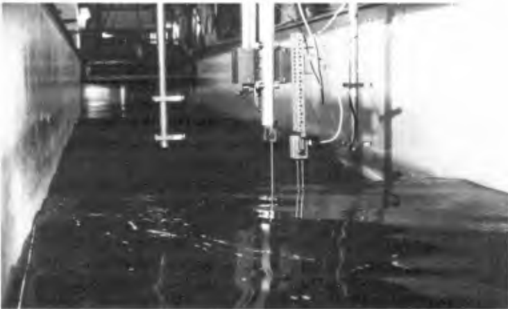
Fig. 3: Set-up of vertical movable frame in the wave flume
