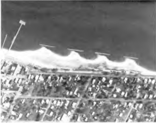
Figure 4. Aerial Photograph of Periodic Tombolo Formation at Central Beach Colonial Beach, Virginia
