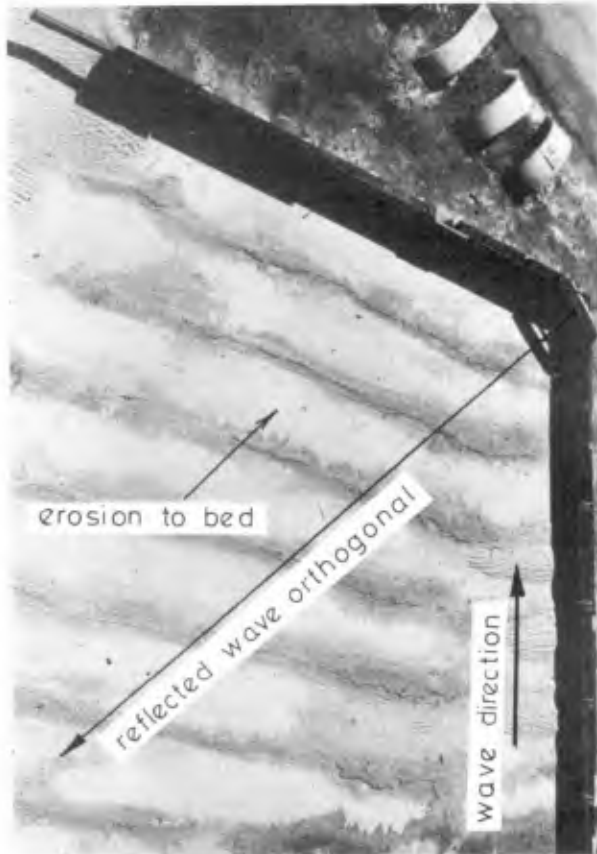
Fig. 7 Differential erosion occurring at quarter crest lengths from the wall.
