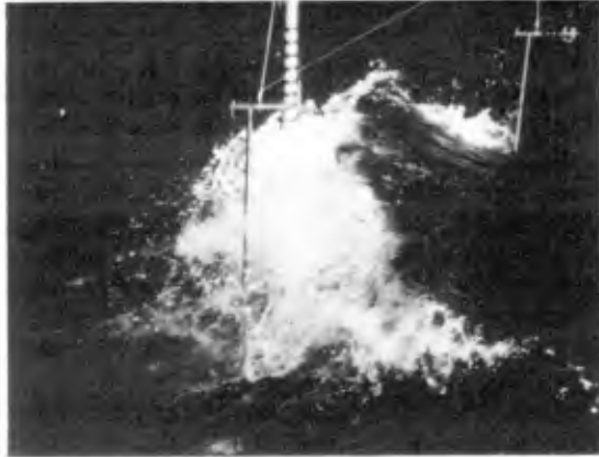
Fig. 8 Short-crested 3-dimensional breaking wave with zero-downcross wave height H_{zd} = 0.692 m and zero-downcross wave period T_{zd} = 1.69 sec. The steepness s_{zd} based on these parameters is 2\pi H_{zd}/g \cdot T_{zd}^2 = 0.155 .
