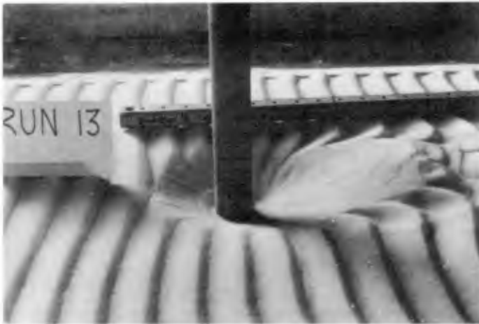
Figure 10. Scour pattern due to random waves and current - Run 13. h=1.167 ft (0.36 m); U_c=.485 fps (0.148 mps); U=.498 ft/sec (0.1518 mps); wave spectrum-Darbyshire; H_{1/3}=.1724 ft (0.053 m); D=.125 ft (0.038 m); S_d=.143 ft (0.044 m)
