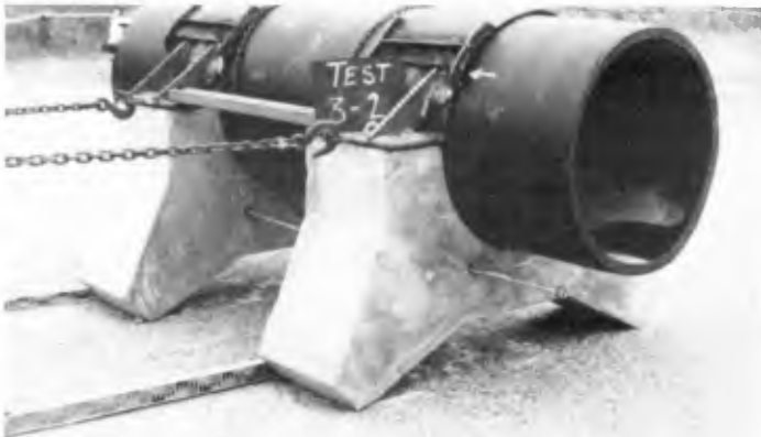
Figure 2: Above-water friction test configuration
