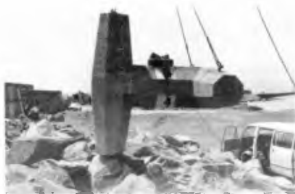
Figure 5: Free-fall tests on 0,5 to 3 t rock.
