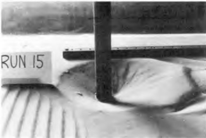
Figure 12. Scour pattern due to random waves and current - Run 15. h=1.167 ft (0.36 m); U_c=.485 ft/sec (0.148 mps); U=.504 ft/sec (0.154 mps); wave spectrum=Jonswap ( T=8 sec); H_{1/3}=.1631 ft (0.050 m); D=.125 ft (0.038 m); S_d=.174 ft (0.053 m)
