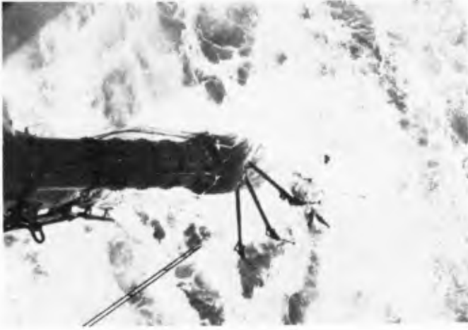
Fig. 2 : Test section clamped on an inclined member of the platform substructure to be seen on extremely low tide water level at storm conditions. Baylor wave staff on the left hand side.
