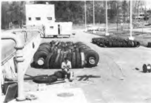
Plate 1. PT-Breakwater before testing at Coastal Engineering Research Center, Ft. Belvoir, Virginia: truck tires/steel pipe on left and automobile tires/telephone pole on right.
