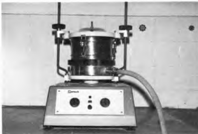
Fig. 4 Testing equipment for the estimation of the effective opening size of geotextiles
