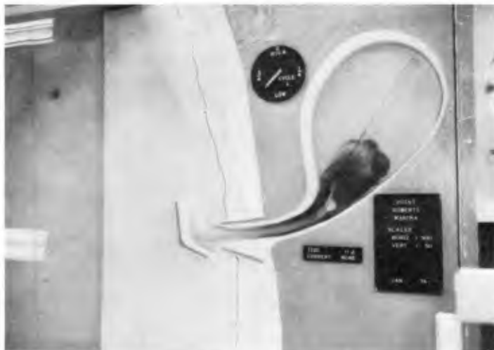
FIGURE 7A MOVEMENT OF DYE FROM ENTRANCE CHANNEL TO BASIN DURING FLOOD TIDE
