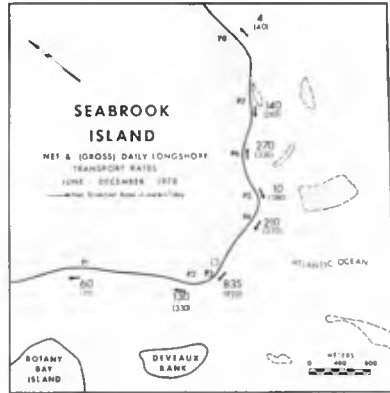
Figure 3. Net and (gross) long-shore transport rates along Seabrook Island based on wave energy flux. Highest net rates at stations 3 and 6 correspond to erosion zones at the time of the survey.
