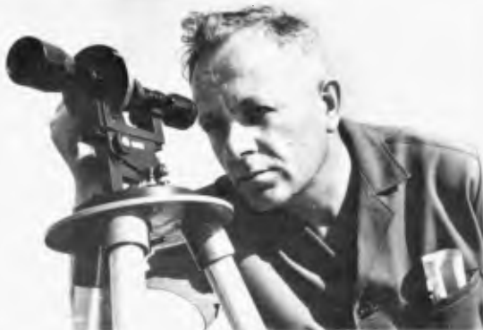
FIGURE 2: WAVE OBSERVATION WITH WAVE CLINOMETER
