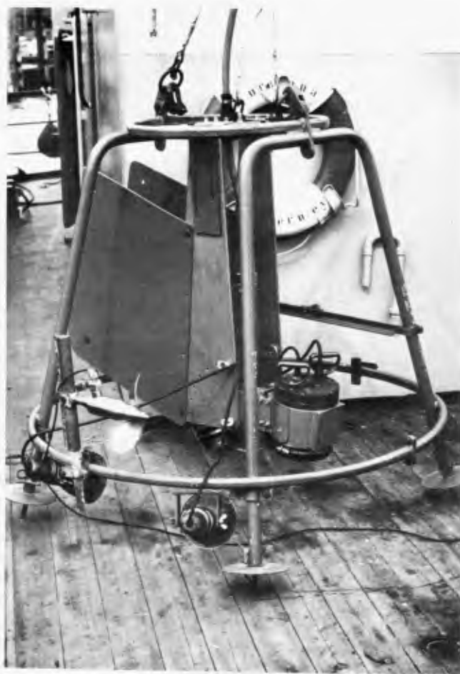
Fig.3 Four-legged support frame on deck
