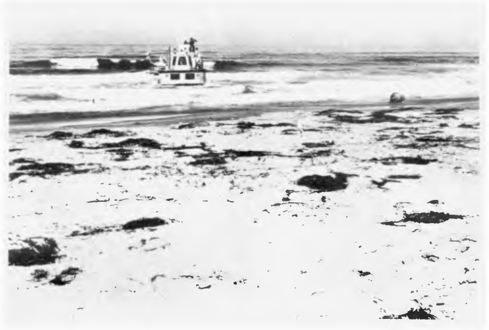
Amphibious LARC XV towing radiation detector vehicle entering surf. The ball-like device is connected to the LARC and the onboard data acquisition system by means of electromechanical cable.
