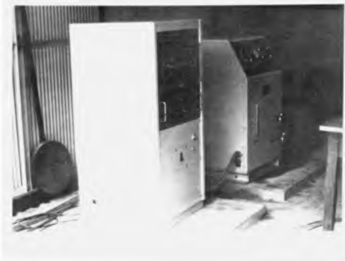
Fig.3 OIL-HYDRAULIC CONTROLLER OF THE TSUNAMI GENERATOR
