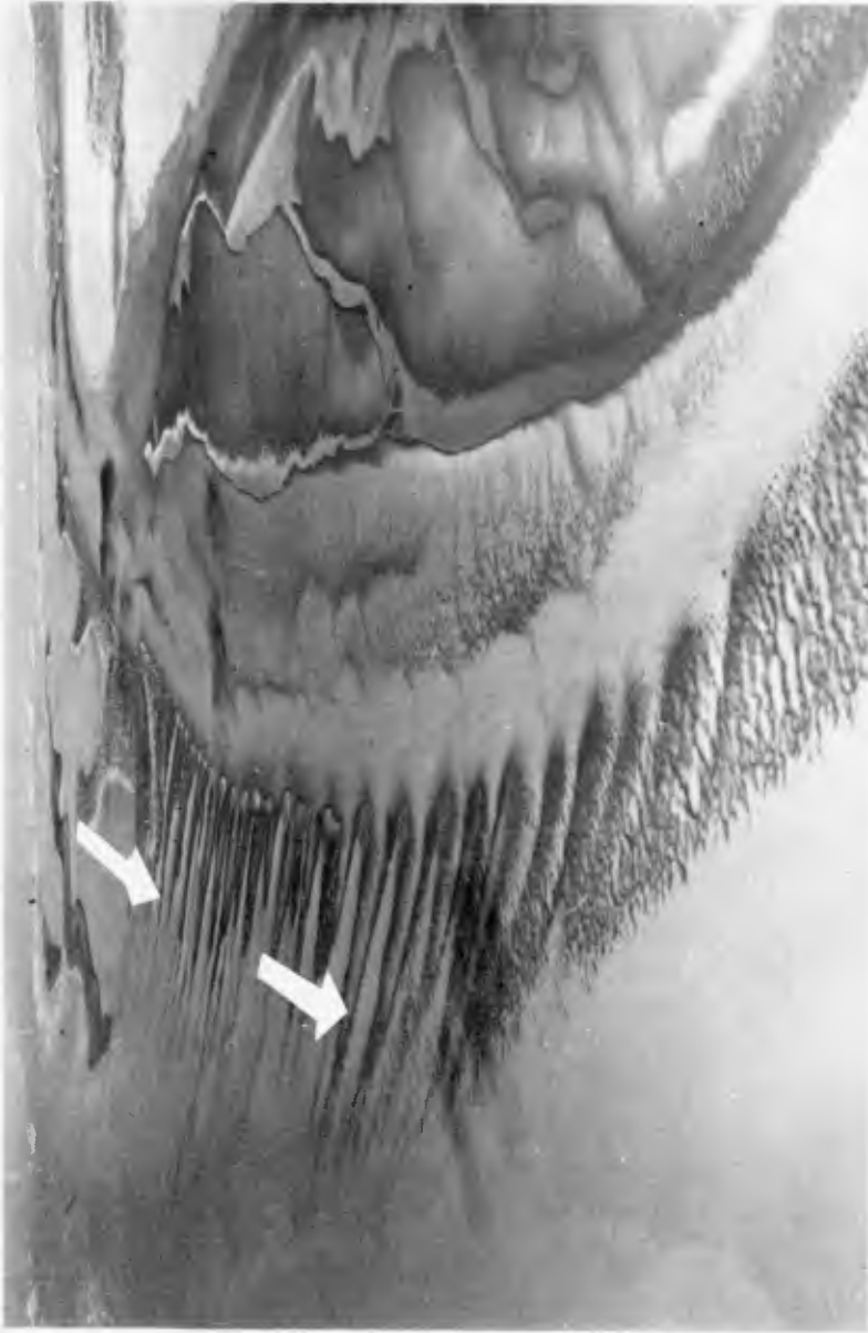
Fig. 8 A flood channel on the downdrift side of an offset inlet, Strawberry Reef, Copper River Delta, Alaska (arrows indicate direction of flood current flow). The view is downdrift (southwest) looking out of the inlet. Flood-oriented sand waves in the middle distance indicate transport of sediment into the inlet. The flank of the main ebb channel is at the lower left-hand corner of the photograph. Photograph taken at low tide in July 1970.
