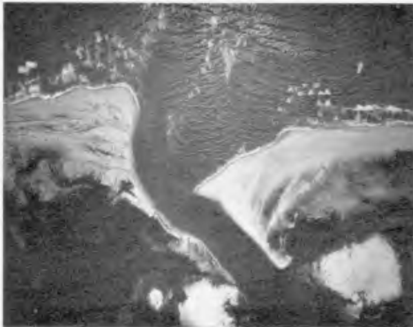
PHOTOGRAPH 2 - VIEW OF CAROLINA BEACH INLET IN 1969. NOTE OFFSET BETWEEN INLET SHOULDERS, AND WAVE REFRACTION PATTERN.
