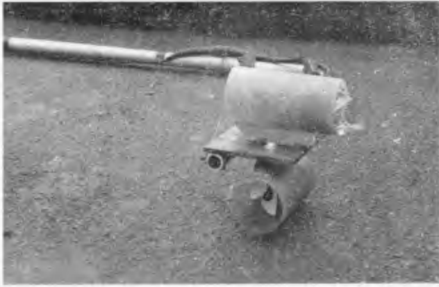
FIG. 4. - PROTOTYPE: ORTHOGONALLY MOUNTED DUCTED IMPELLER CURRENT METERS
