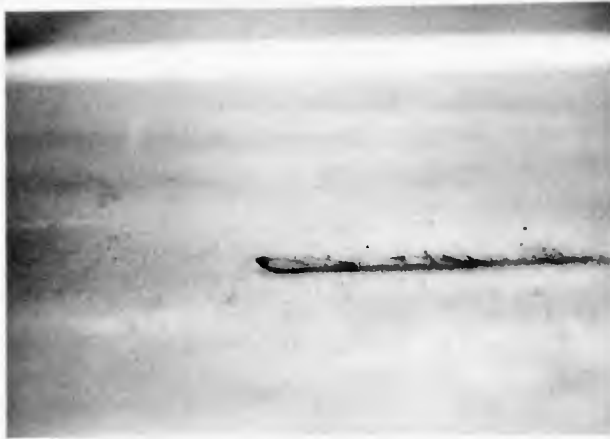
Figure 7. Boundary layer obtained with injected dye on a rough boundary.
