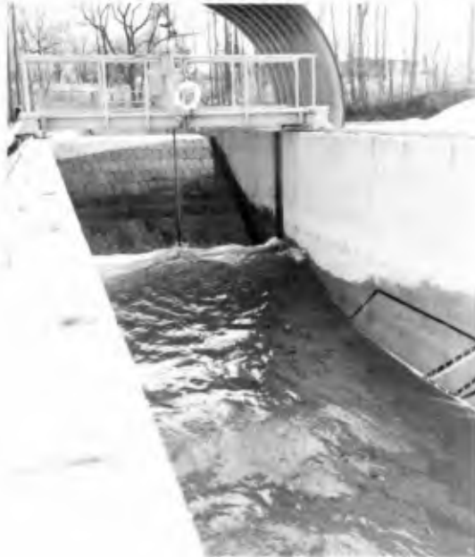
Fig. 7. Concrete block revetment in large wave tank.
