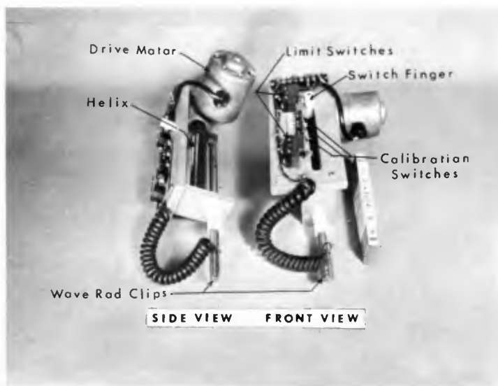
Fig. 5. Automatic wave rod calibration unit.
