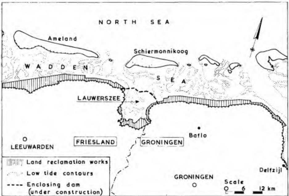
Fig. 2. Eastern Wadden Shallows, with land reclamation area.
