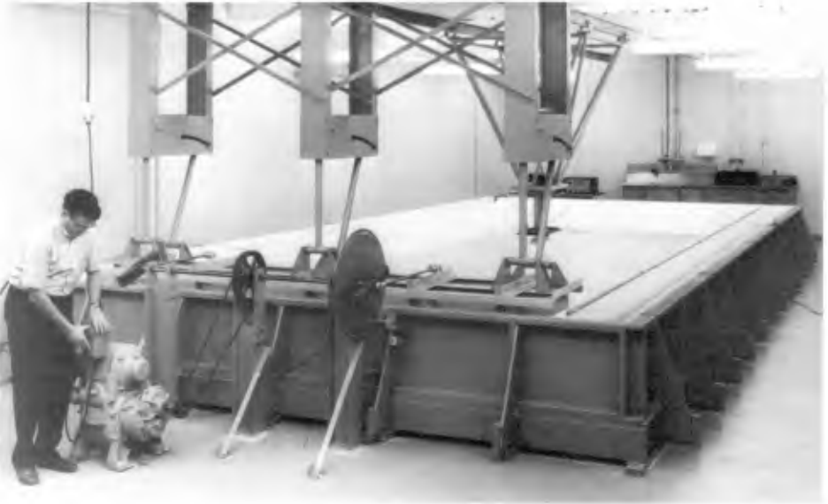
Fig. 3. Overall view of wave basin and wave generator.
