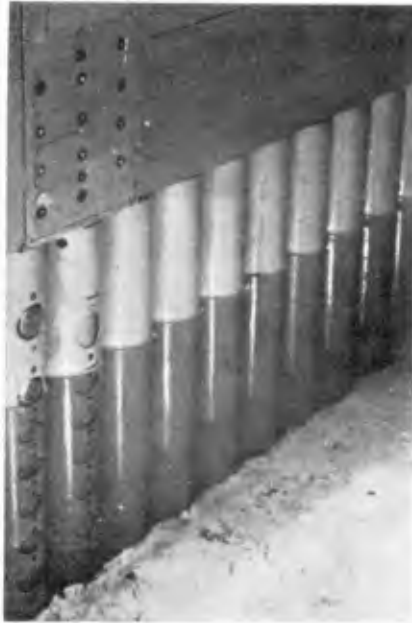
Fig. 1. Model of the steel-pipe breakwater.
