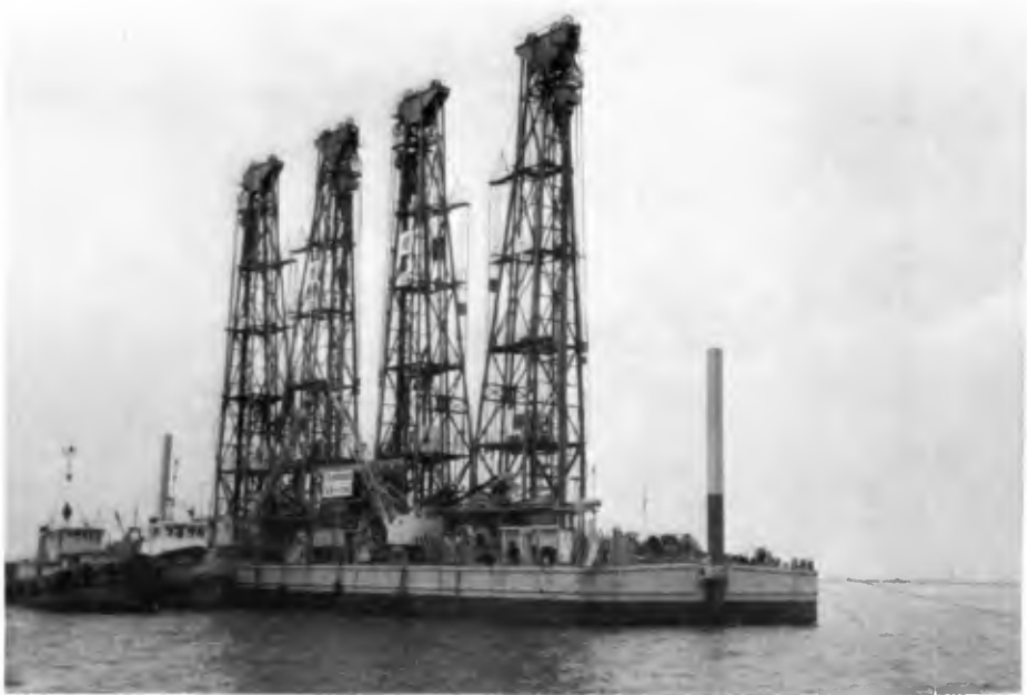
Fig. 18. "SORYU" craft for sand piling.
