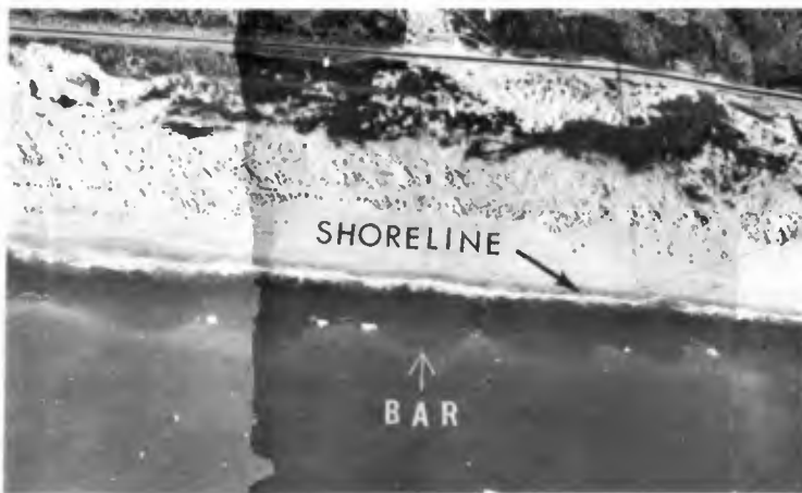
Fig. 3. Aerial photograph showing sand wave phenomena approximately 5 miles south of study site, taken December, 1957 (Courtesy of Cape Hatteras National Park Service).
