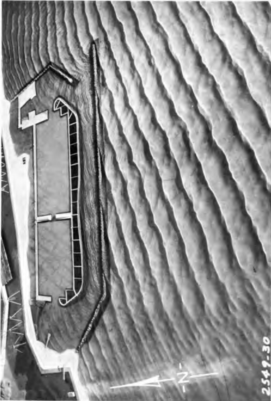
Fig. 7. Wave patterns, 9.0-sec waves 13 ft. high from S5°E. West breakwater crown at +18 ft. mllw. (U.S. Army Corps of Engineers, Waterways Experiment Station)
