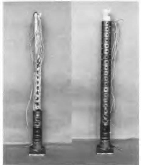
Photo. 2. Pile for the measurement of moment distribution.
