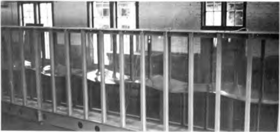
Fig. 2. Typical portion of the test section (Dimensions: channel cross section, 74-1/2" high x 35-1/2" wide). 1e)
