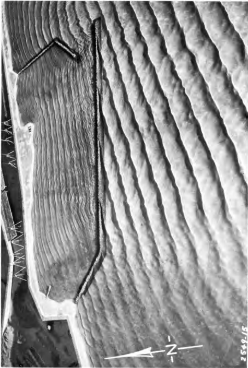
Fig. 6. Wave patterns, 9.0-sec waves 13 ft. high from S5°W. West breakwater crown at +18 ft. mllw. (U.S. Army Corps of Engineers, Waterways Experiment Station).
