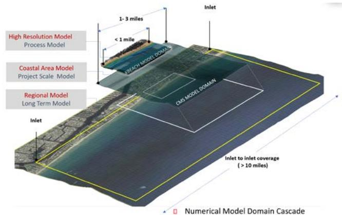
Figure 1 - Model cascade from process modeling to setup large scale contour line regional model and assess equilibrium planform
