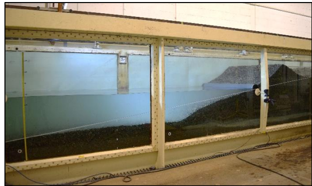
Figure 3 - Beach profile change after beach equilibrium was met with a single log placed at the still water level. The white line indicates the original 8:1 (H:V) beach profile.
