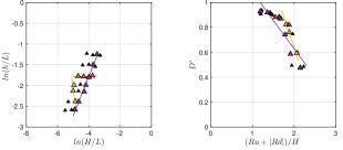
Figure 1. (a) Experimental space [H/L vs h/L] with three experimental testing techniques: (orange) constant h/L; (yellow) constant H/L or Ir; and (purple) varying h/L and H/L. (b) relationship between the bulk dissipation and the total excursion.
