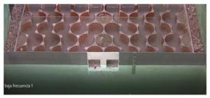
Figure 1 - Scale model example of an ARJ-R structure with long dissipative circuits made of circular cells with two frontal openings to the basin.
