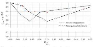
Figure 2 - Reflection coefficient of the ARJ-R structures related to the relative width of the dissipative chamber
