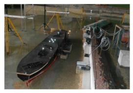
Figure 2 - Ship's model with moorings instruments and optical point trackers
