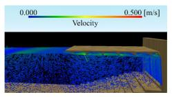
Figure-2 calculated flow velocity near the pier
