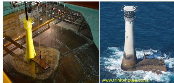
Figure 2 Tests in the Ocean Basin, University of Plymouth
