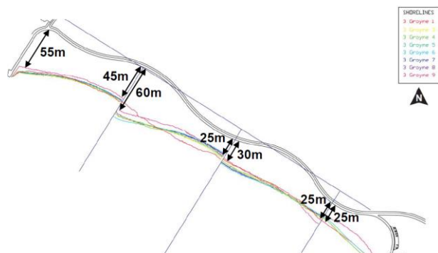
Figure 7 - Alignments of the beach compartments predicted by the mobile bed model
