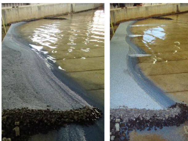
Figure 6 - Mobile bed model of the eroded beach (left) and the beach stabilised with groynes (right)
