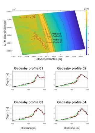
Figure 1 - 1D and 2D model validation results at Gedesby. Above: Location of Gedesby profiles. Below: Profile graphs of Gedesby profiles. Green: Before the storm. Red: Measured profile after the storm. Dashed black: 1D model result. Filled black: 2D model result.
