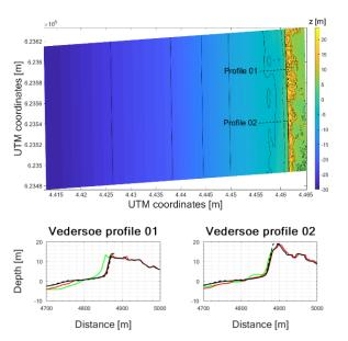
Figure 2 - 1D and 2D model validation results at Vedersoe. Above: Location of Vedersoe profiles. Below: Profile graphs of Vedersoe profiles. Green: Before the storm. Red: Measured profile after the storm. Dashed black: 1D model result. Filled black: 2D model result.
