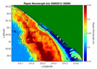
Figure 1 - Plot of the modeled ripple length in a domain off the coast of Panama City, FL.
