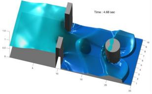
Figure 1 - Snapshot from a dambreak problem showing sharp shock fronts - computed by the GPGPU code.
