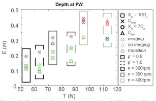
Figure 2. Results of maximum eroded depth (E) at t = 30min for all the experiments. Thrust (T) is calculated per each propeller according to (eq.1).
