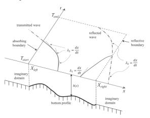
Figure 1 - An illustration of characteristics of the onedimensional wave propagation in x – t domain.
