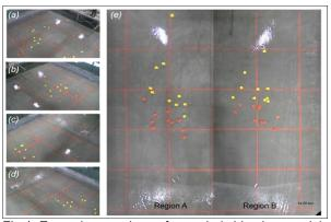
Fig.1: Example snapshots of recorded video images (a) to (d) A raw video images. (e) A rectified and merged image.
