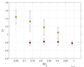
Fig 2: Normalized mean longitudinal distance,  $\overline{D}_{\chi}^{*}$  of HDPE and wood and debris as a function of  $SG_{g}$ . Vertical bars indicated a 95% confidence limits (c.l).
