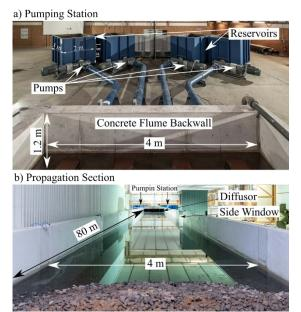
Figure 1. a) Pumping station including four rotary lobe pumps, reservoirs and pipes. b) Concrete flume, view directed towards the pumping station.
