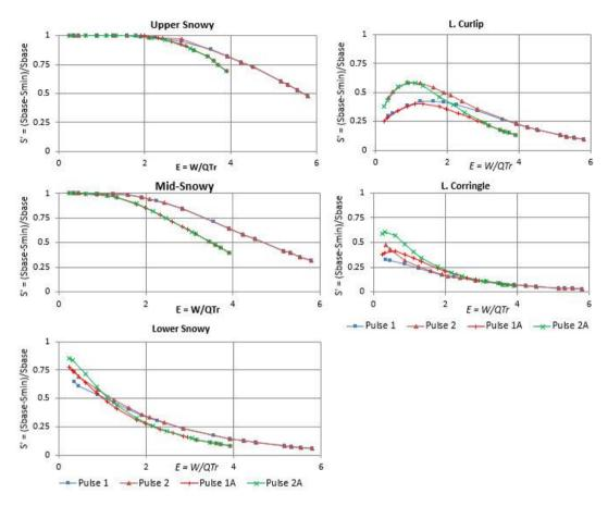
Figure 6. Minimum salinity (normalised by  $S_{base}$ ) as a function of estuary flushing parameter, *E*. Left hand plots are for main Snowy River channel, right hand plots are for tributaries
