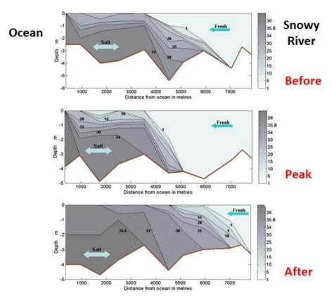
Figure 3. Long profile salinities for the 2011 EFR at stages of the flow release.
