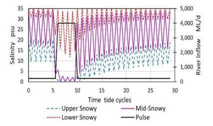
Figure 4. Inflow hydrograph for Pulse 1 of duration 4 tide cycles, with salinity histories at 3 sites along the Snowy River channel (high and low tide values).
