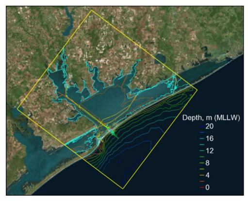
Figure 5. CMS model domain and bathymetry.
