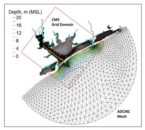
Figure 4. ADCIRC mesh and CMS model domain (red box area).
