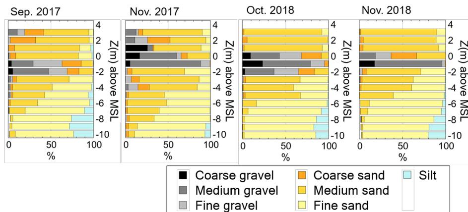
Figure 10. Depth changes in composition of sea bed material before and after T1721.
