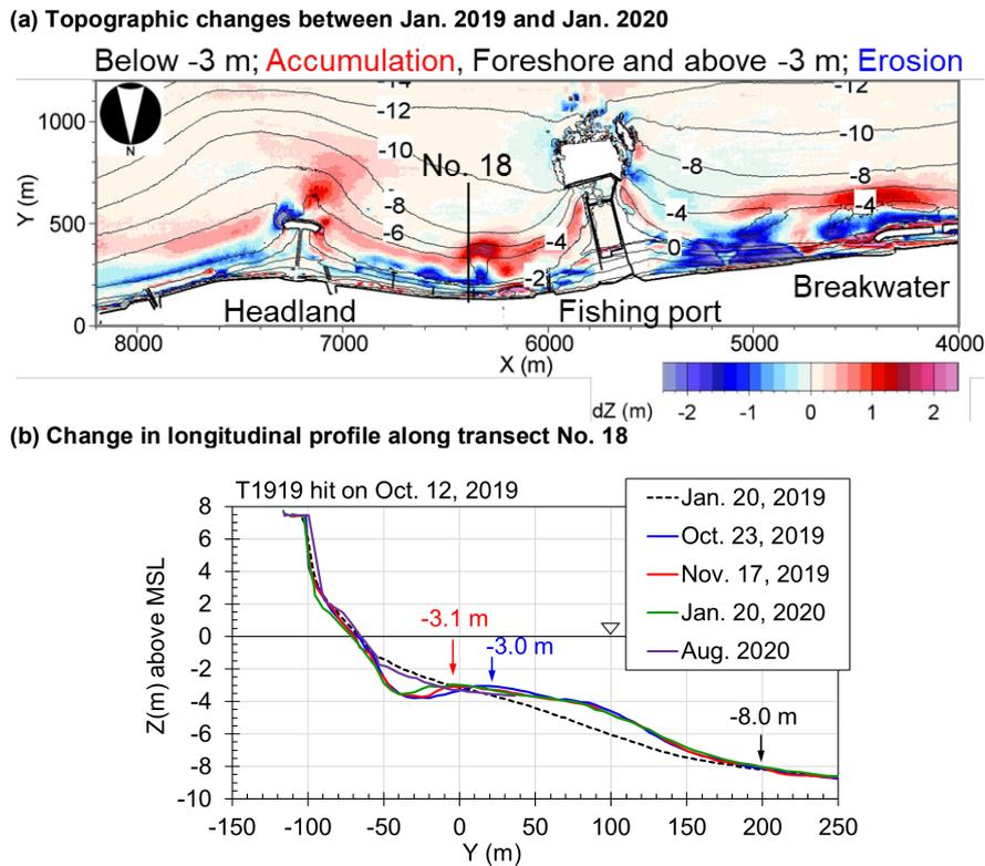
Figure 11. Topographic changes between January 2019 and January 2020 and change in longitudinal profile along transect No. 18.
