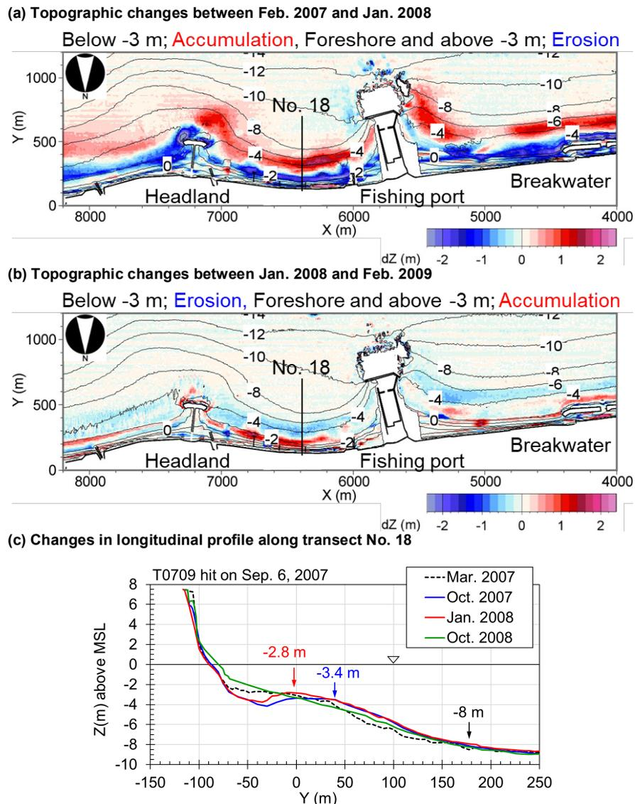
Figure 5. Topographic changes immediately after T0709 hit on September 6, 2007 and change in longitudinal profile along transect No. 18.
