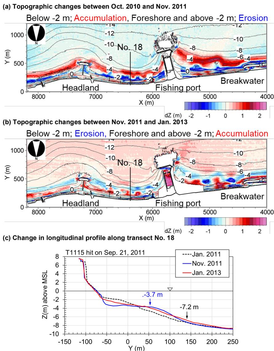
Figure 6. Topographic changes immediately after T1115 hit on September 21, 2011 and change in longitudinal profile along transect No. 18.
