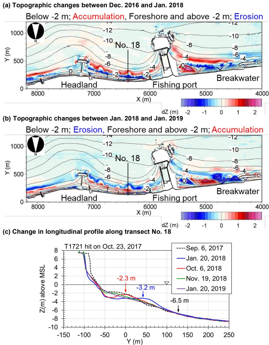
Figure 8. Topographic changes immediately after T1721 hit on October 23, 2017 and change in longitudinal profile along transect No. 18.
