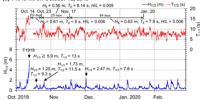
Figure 3. Wave height and wave period during T0709, T1115, T1721, and T1919 and in subsequent periods after each typhoon event.
