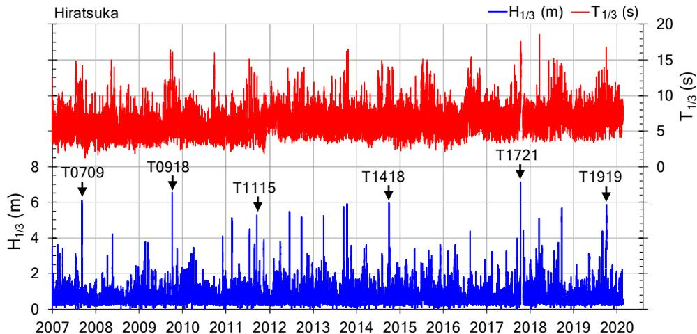
Figure 2. Wave height and wave period during six typhoon events since 2007 measured at Hiratsuka wave observatory.
