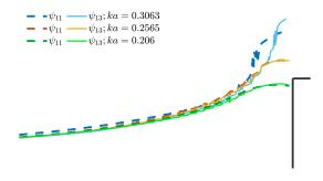
Figure 5: Form of the overshooting jets under different wave steepness but same impulse parameter at the vertical sea defence.  $\psi_{11}$  and  $\psi_{13}$  refers to the first and the third of the three consecutive wave cycles.
