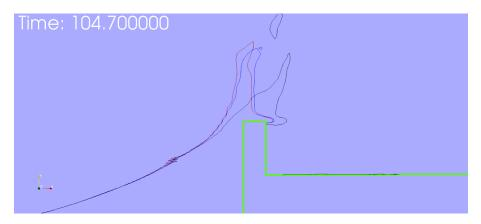
Figure 6: Overshooting jets in Type A and Type B overtopping. The case in red line shows the jet in Type A with zero wind speed, whereas, the case in blue is for Type A with low wind speed in Type A. The profile in black shows the overshooting jet under wind speed in Type B.
