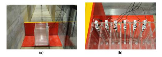
Figure 2: (a) Tank after the defence model to collect overtopping water and (b) the dip sticks inside the tank compartments.
