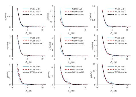
Figure 3: Overtopping rates measured across distance from the sea defence crest.
