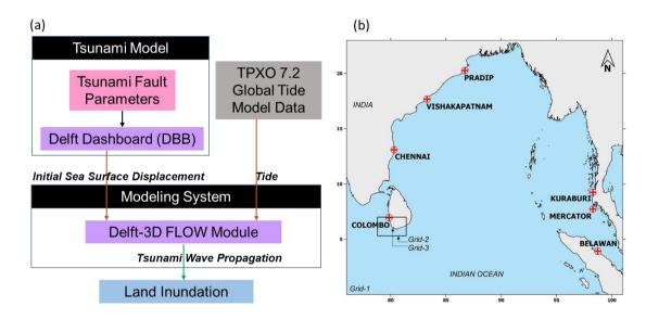
Figure 2: (a) Modeling framework (b) Computational domain with tide gauges used to calibrate the model
