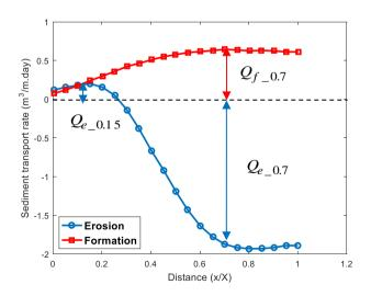
Figure 4. Sediment transport rate by Suzuki and Mochizuki (2014).
