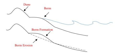
Figure 3. Schematic diagram of berm formation and erosion
