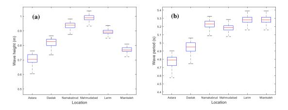
Figure 2. Wave condition for each coastal region of Caspian Sea; (a) significant wave height and (b) mean wave period.
