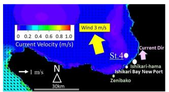
Figure 16. Profile of current velocity when wind direction was SE (5hours after staring simulation)
