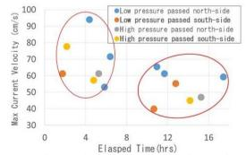
Figure 12. Relationship between maximum velocity and reach time after starting wind direction changed
