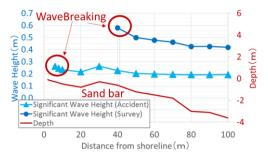
Figure 9. Shallow water deformation of Ishikari-hama beach (Accident and Field Survey)
