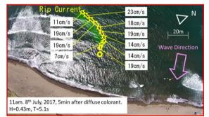
Figure 11. Velocity profiles of Rip Current (at point 1 in Figure 2)
