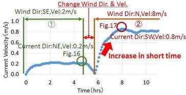
Figure 15. Simulation result of time change of current velocity due to change of wind condition (Ishikarihama, 11<sup>th</sup> August, 2016)
