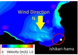
Figure 14. Profile of current velocity when field survey
