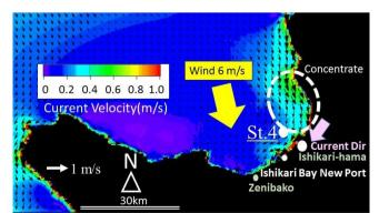
Figure 17. Profile of current velocity when wind direction was NNW (8hours after staring simulation)
