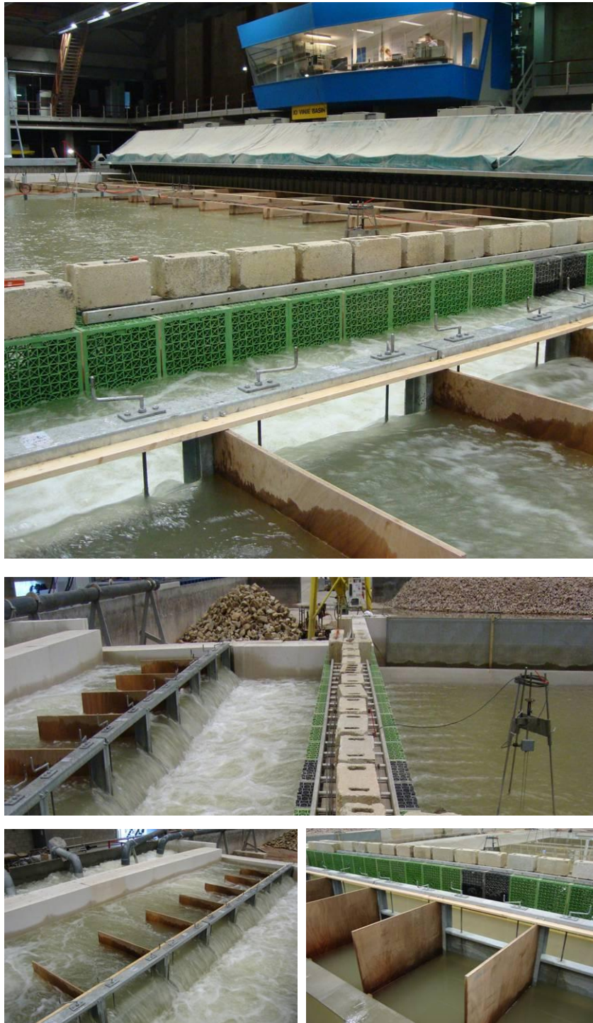
Figure 3. Pictures of the inflow (a system of weirs and flow dividers).
