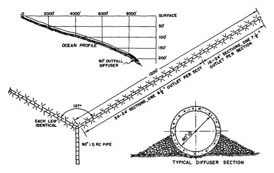
Fig. 11. Diffuser for 90 inch diameter outfall Los Angeles County Sanitation Districts No. 3
