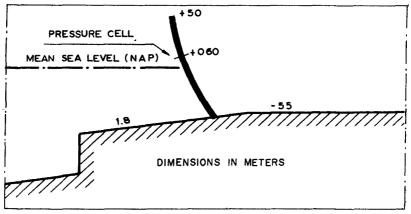
Fig. 1. Forward inclined face.
