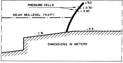
Fig. 2. Backward inclined face.
