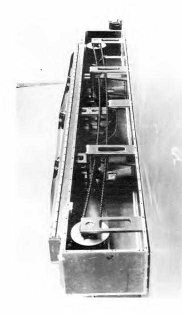
Fig. 4 View of the moving boundary mechanism.
