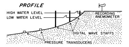
Figure 1. Schematic diagram of sensor array used for measuring direction and flux of wave energy (after Koontz and Inman, 1967, Fig. 16) Cross-spectral analysis shown in Figure 2 is from a longshore pair of such an array.
