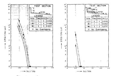
Fig. 1-a, h/Ho = 0 Relation between 2NQ/(HoLo) and hc/Ho with a parameter of Ho/Lo
