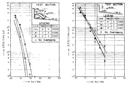
Fig. 4-a, h/Ho = 1.5 Fig. 4-b, h/Ho = 1.5 Relation between  $2\pi Q/(HoLo)$  and hc/Ho with a parameter of Ho/Lo
