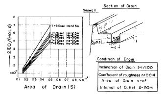
Fig. 17 Relation between wave overtopping and the capacity of drain.
