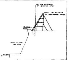
Fig. 11 Facilities of field observation of wave overtopping at Sakata Coast.
