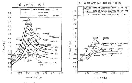
Fig. 6-a Fig. 6-b Relation between hc/Ho and h/Lo with a parameter of 2TQ/(HoLo)
