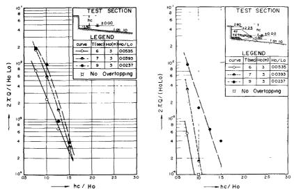
Fig. 2-a, h/Ho = 0.5 Relation between 2RQ/(HoLo) and hc/Ho with a parameter of Ho/Lo
